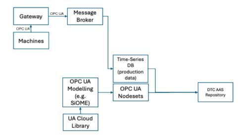
With the OPC Foundation Cloud Initiative, best practices are used to create a cloud reference architecture, increasing standardized data sharing and cloud-optimized, OPC UA-enabled services. In addition, a mechanism to model Asset Administration Shells (AAS), with the OPC UA modelling language, has been created.
