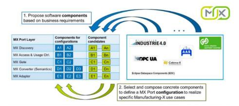
These layers can be implemented by using different protocols & technology components. Each defined combination of components is called a configuration (Hercules, Orion – see below).
