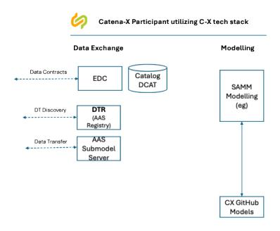
From a data exchange perspective, Catena-X utilizes 3 core components, which are typically referred to as "Enablement Services":
