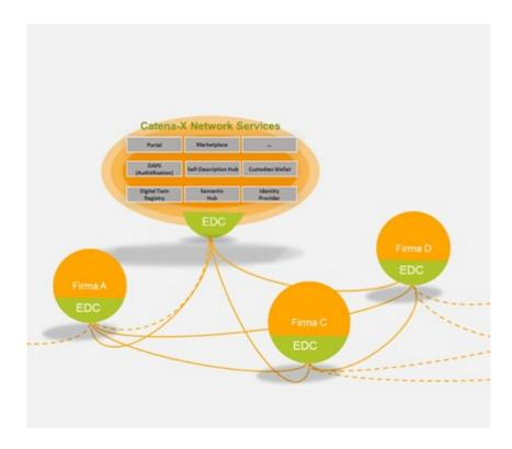
The Eclipse Data Space Connector (EDC) (see standard CX-0018) defines access and usage policies for the different digital twins and aspects of the digital twins.
