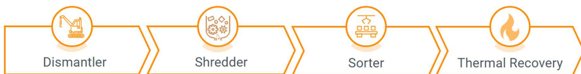
Figure 5 Current process steps for recycling of non-metallic parts of seats.
