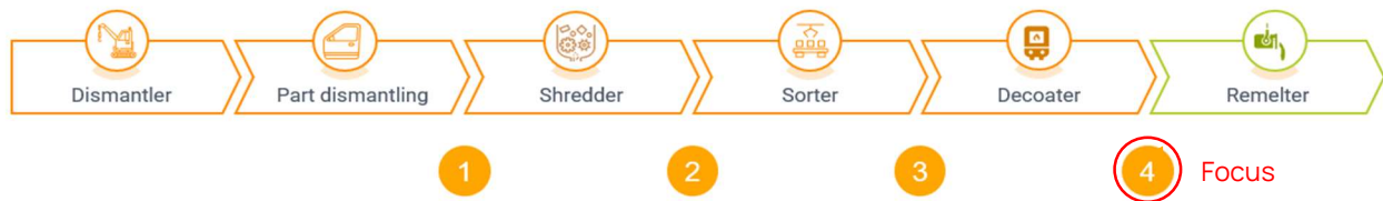
Figure 7 Process steps for non-iron metal recycling with data handover steps.
