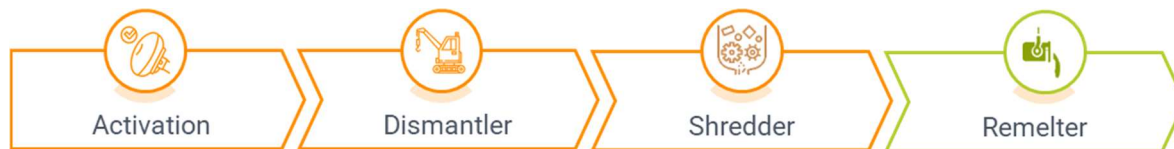
Figure 4 Current process steps for recycling of airbags.
